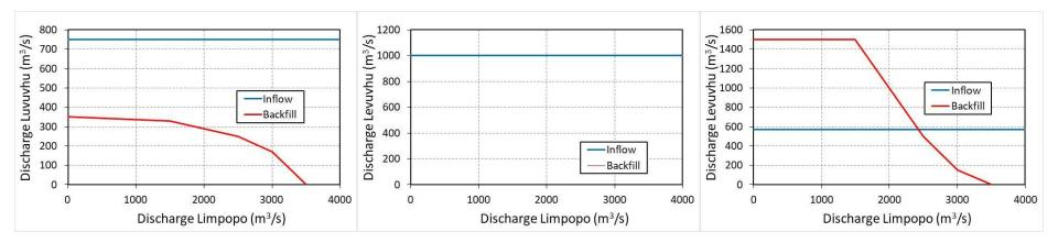
The combinations of discharge in the Luvuvhu and Limpopo Rivers that breach the levees and flood the floodplain to fill the Nwambi and Mambvumbvanyi (left), Hapi (center) and Tlangelani (right) pans.
