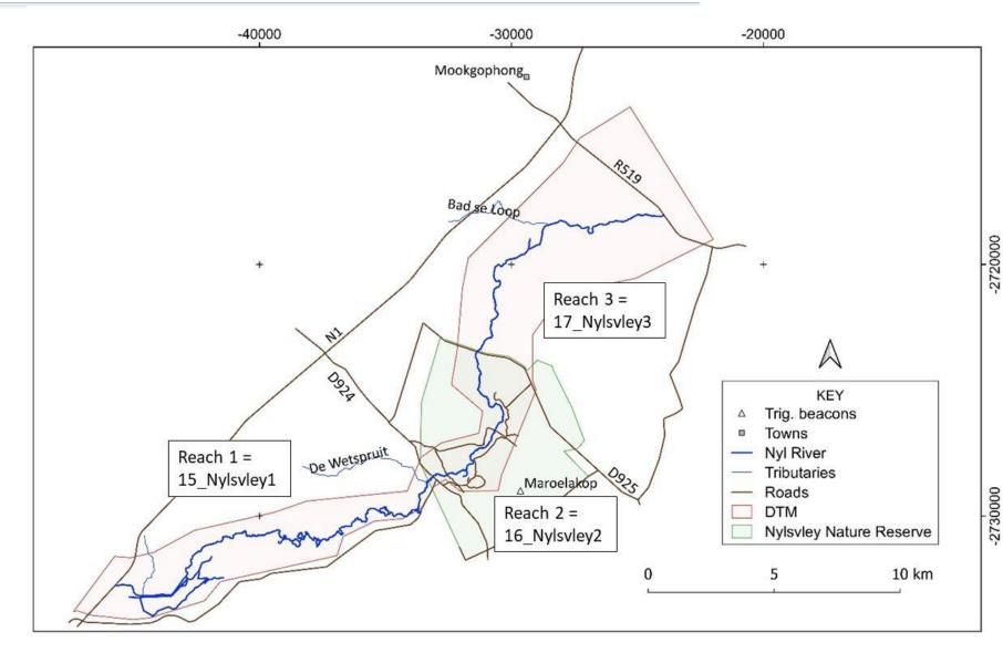
Three 2001 HECRAS sub-models were designed, one per reach using a multitude of cross sections.
